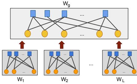
Fig. 2. A two-level error correcting neural network.
